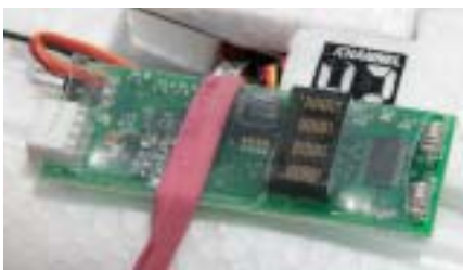
Above: The ZLog Recording Altimeter with its USB interface module. Below: The ZLog was simply strapped to the side of the Multiplex Space Screamer during flight testing.
