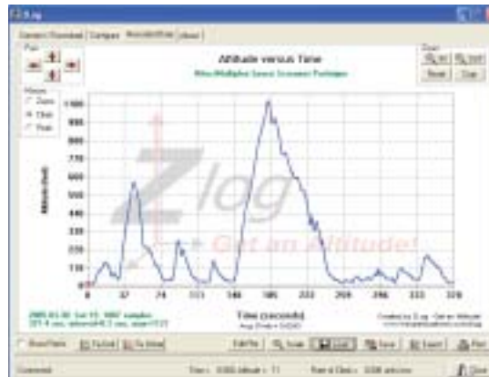
Here is the ZLog graph of an entire flight with the Space Screamer. Many of the display parameters are adjustable to suit your preferences.
