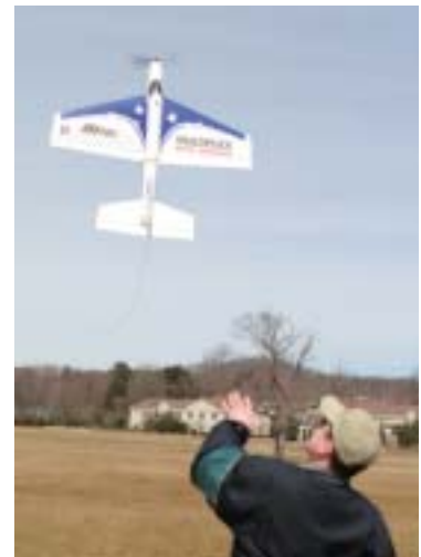
The Multiplex Space Screamer easily will climb vertically out of your hand. The ZLog tracked a 1,000-foot, 30-second climb in the midst of one flight as shown in the graphs.
