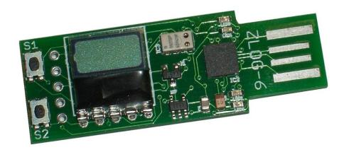
The Hexpert Systems ZLog-6 recording altimeter (Z6R) provides a lightweight, compact device for highly accurate measurement of altitude (pressure altitude) in your application. It was designed specifically for use onboard a radio controlled (R/C) aircraft, but should be useful in other applications.
