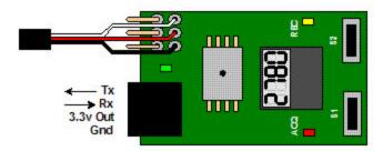
The serial interface operates at 115200 baud, 8 data bits, 1 stop bit, and no parity. The output can be toggled on or off by sending Zlog a lower-case 'L' character (hex 0x6C). Data is output as a 16-bit binary value, most significant byte first. The value represents the current altitude in the units as currently configured in Zlog. The value will be output at the configured rate.
